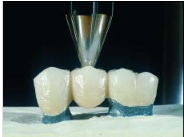
Fig. 5. A loading rod was positioned in the center of the occlusal surface of the all-ceramic pontic and loaded until fracture of the test bridge occurred.
